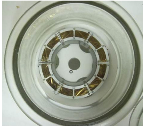
Figure 2: Rotating target cassette in assembly, used for uniform irradiation of the target material.
