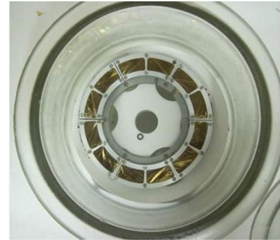
Figure 2: The photo of the rotating target cassette in assembly. 6 packs, 2 windows at 14 mm width each. Target material- ^{242}\text{Pu} in oxide state put on the Ti 2\ \mu\text{m} thick foil
