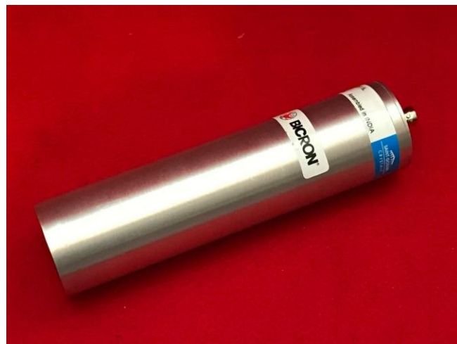
Figure 9 NaI detector configuration
