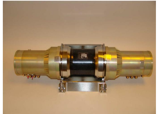
Figure 3 BGO detector configuration
