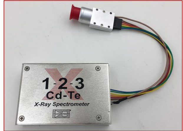
Figure 15 CdTe detector configuration
