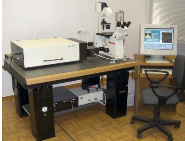
Figure 8. Solar TII Raman spectrometer setup.
