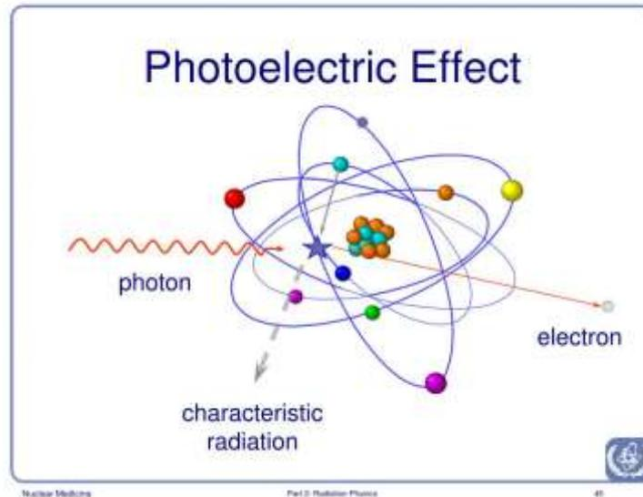
Fig. 7. Schematic of the photoelectric effect.
