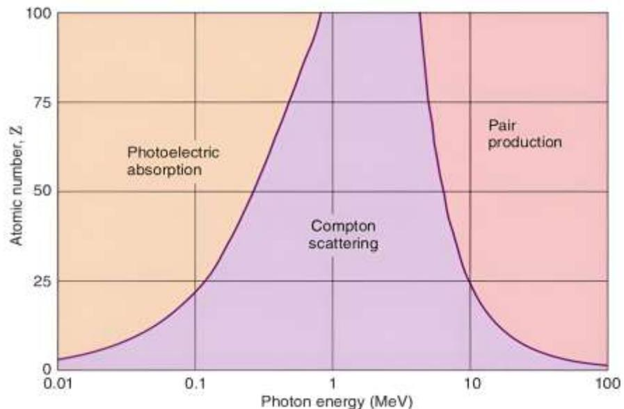
Fig. 6. Main photon interactions versus photon energies for different atomic number [11].
