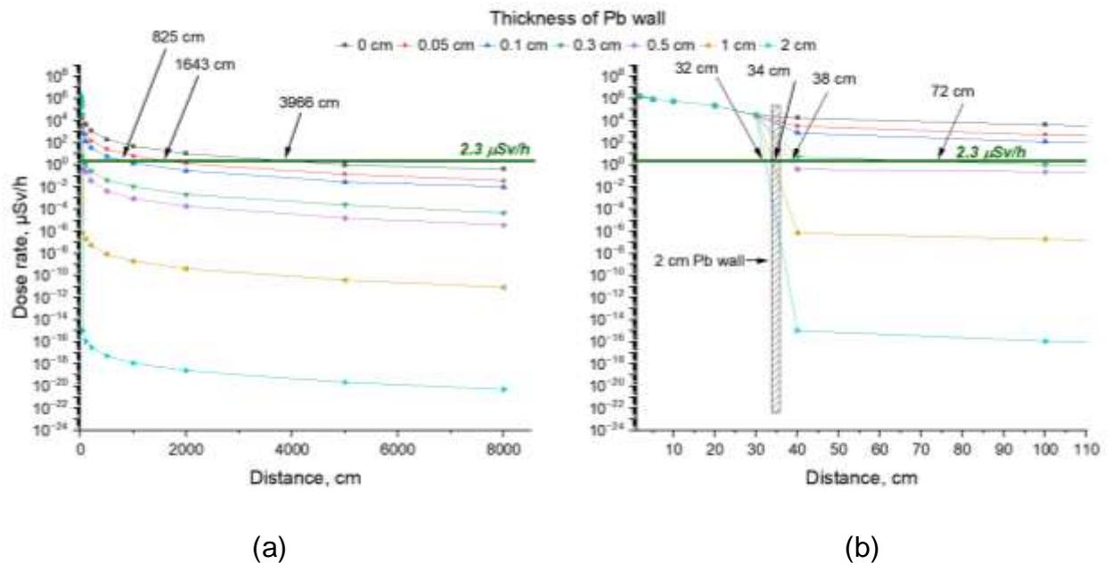
Fig. 12. Dependency of dose rate vs distance from X-ray source in CT setup: (a) - full view, (b) - expanded view of the low distances region.
