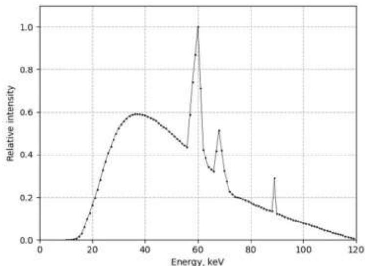
Fig. 11. X-ray tube spectrum with tungsten cathode.
