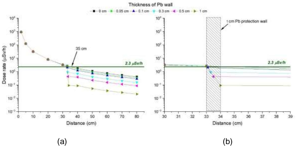
Fig. 14. Dose rate dependence on distance to  $^{131}\text{I}$  gamma source in SPECT setup: (a) - full view, (b) - expanded view of the low distances region.
