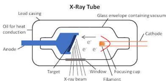
Fig. 4. Production of X-Rays in a Roentgen tube [7].
