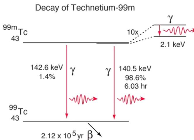
Fig. 3. Technetium-99m decay scheme [5].
