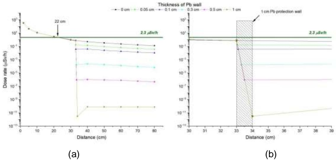
Fig. 13. Dose rate dependence on distance to  $^{99m}\text{Tc}$  gamma source in SPECT setup: (a) - full view, (b) - expanded view of the low distances region.
