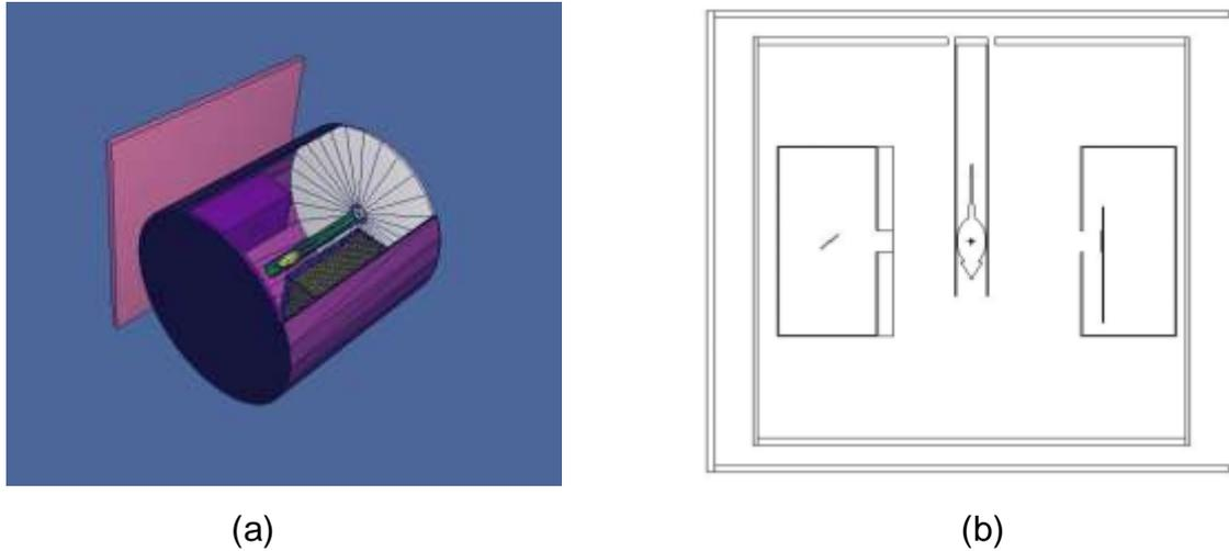
Fig. 10. The geometry of SPECT/CT scanner. (a) - 3D view, (b) - overhead 2D view.
