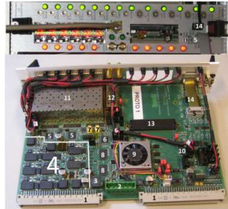
Figure 3. Front and side view of ALICE Trigger Board (ATB). The following components are visible (see in the text for details). 1: VME 6U power supply connector 2: ELMAbox power supply connector 3: power decoupling - inductance 4: DC-DC converter 5: PMbus 6: PLL 7: Clock from PLL 8: DDR4 9: FPGA 10: Flash memory 11: two six-fold SFP+ 12: single-fold SFP+ 13: FMC 14: JTAG-microUSB
