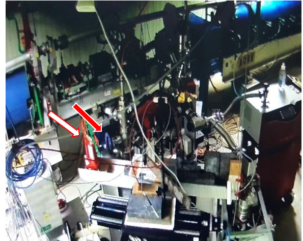
Figura 6. Irradiation post. A red arrow indicates the exit window and a white arrow indicates the sample holder.
