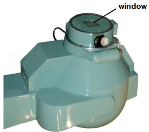
Figure 3. Position of the chamber head during irradiation. The window in which the samples were directly placed is indicated.
