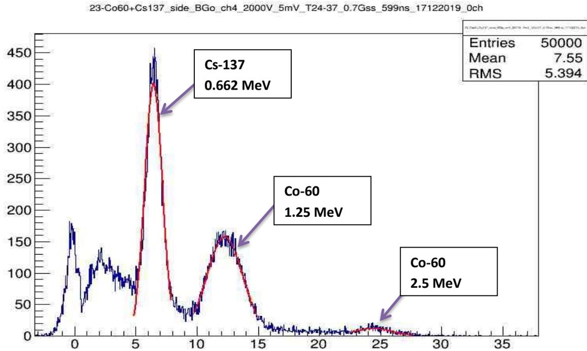
**Figure 4.** Cs-137 and Co-60 spectrum from measurements with BGO detector at 2000 V and threshold voltage of 5 mV
