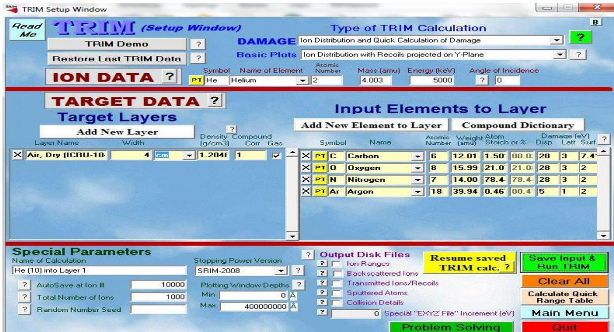
**Figure 15** Parameters used for the simulation of an alpha particle in air using TRIM
