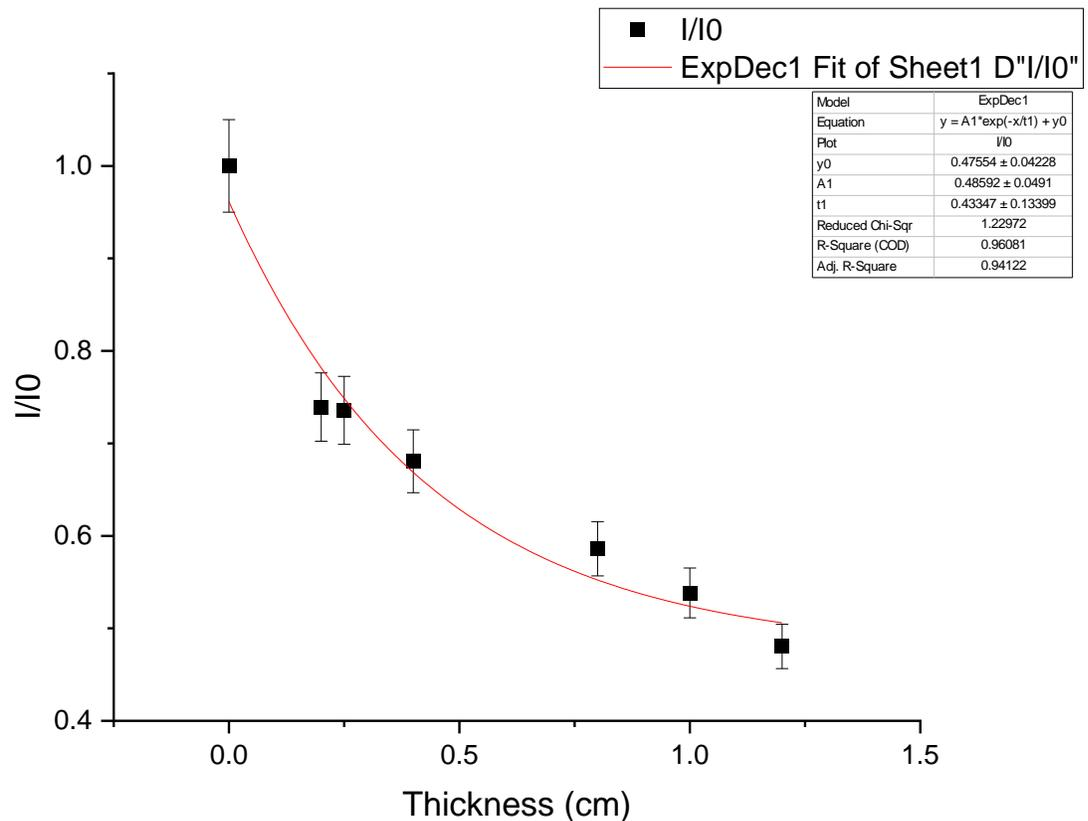
**Figure 12.** Determination of attenuation coefficient for Cu
