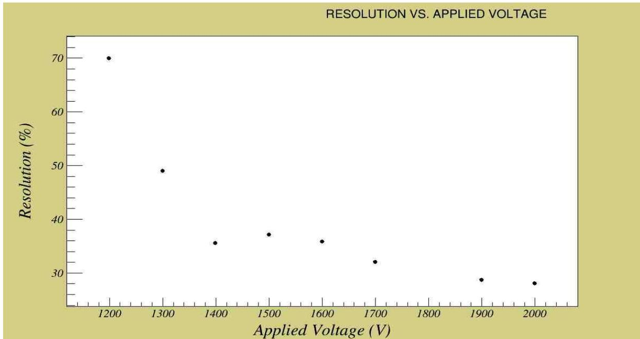
**Figure 3.** The relation between resolution and applied voltage for a BGO detector
