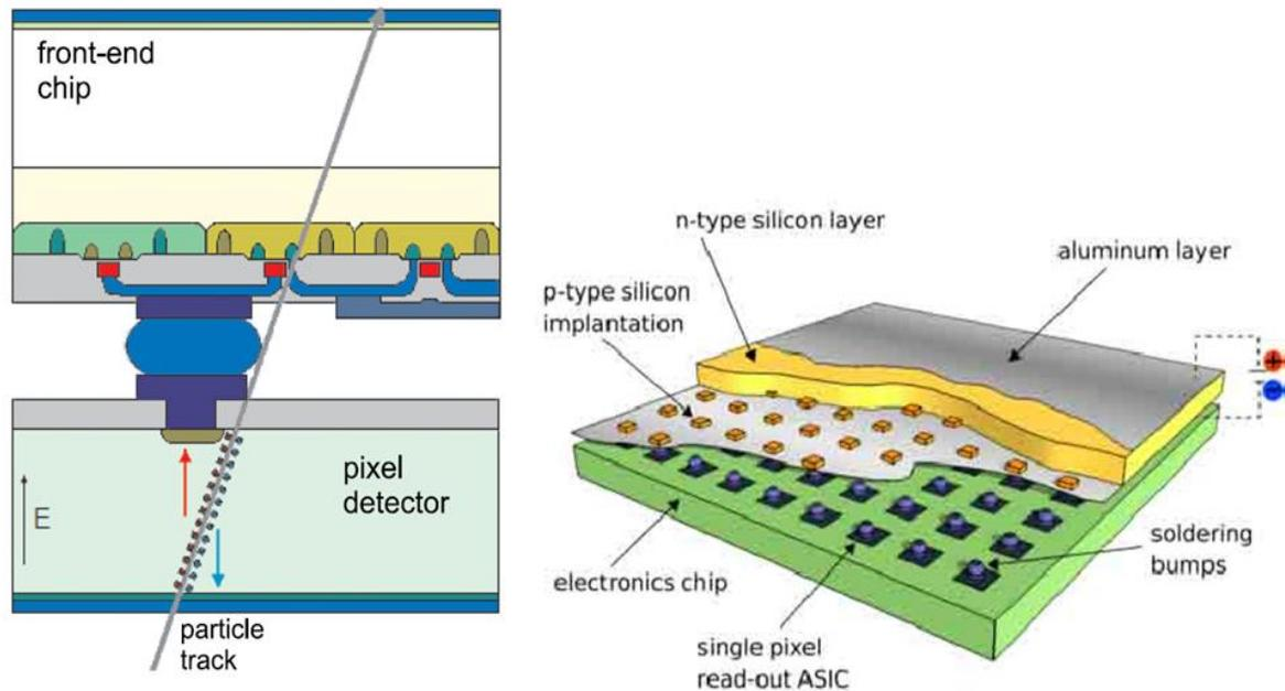
**Figure 17.** Pixel detector
