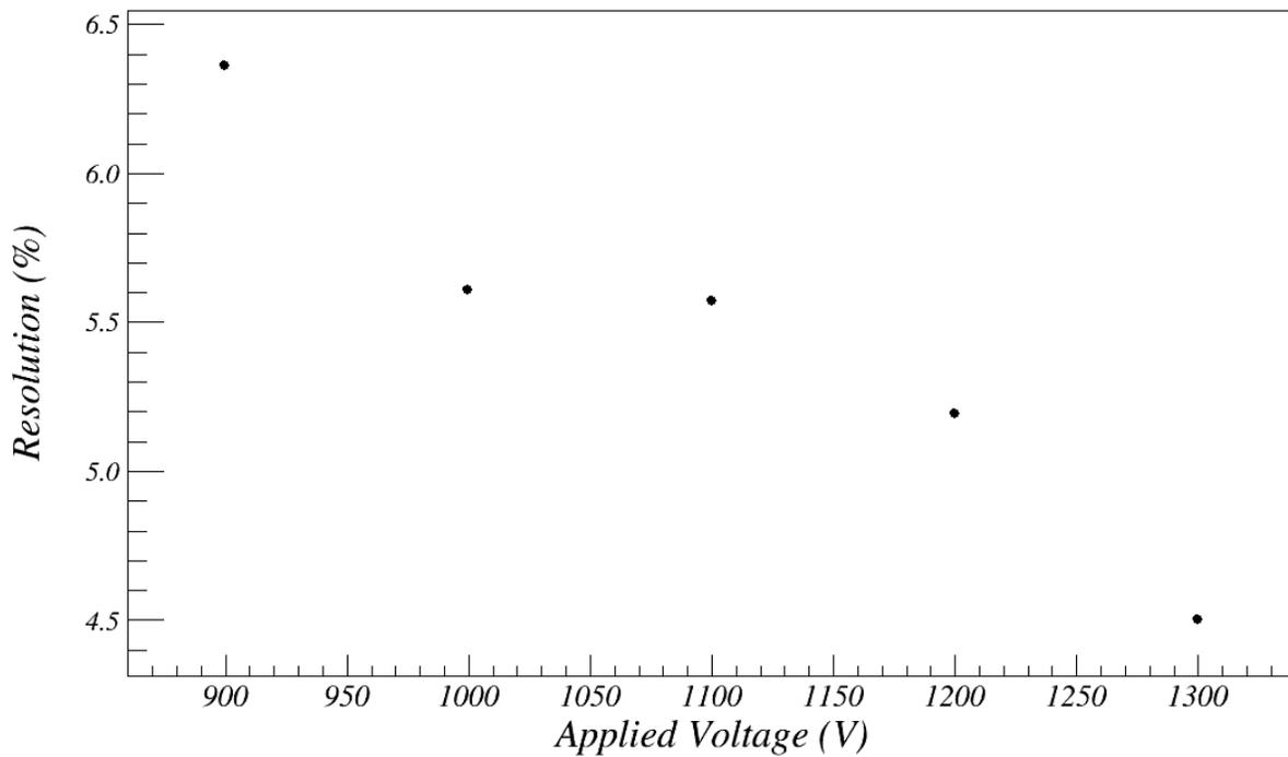
**Figure 6.** Graph showing the relationship between applied voltage (V) and the resolution (%) of a NaI detector.
