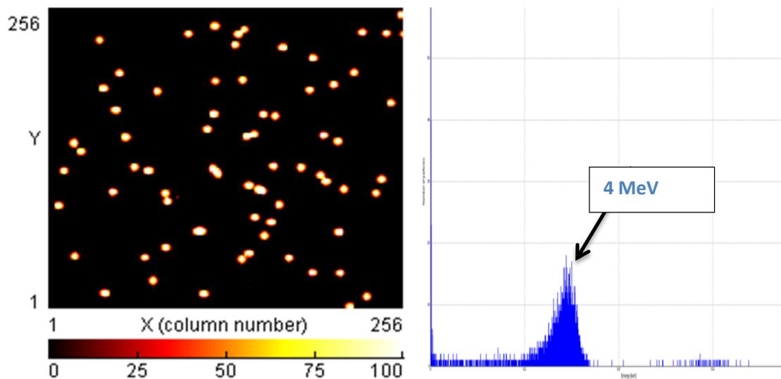
**Figure 18.** Absorption of alpha particles in the air  $d=0$  cm
