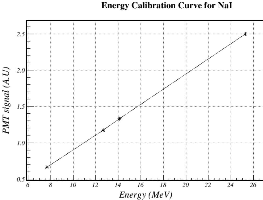
**Figure 9.** Graph showing the energy calibration of a NaI Detector
