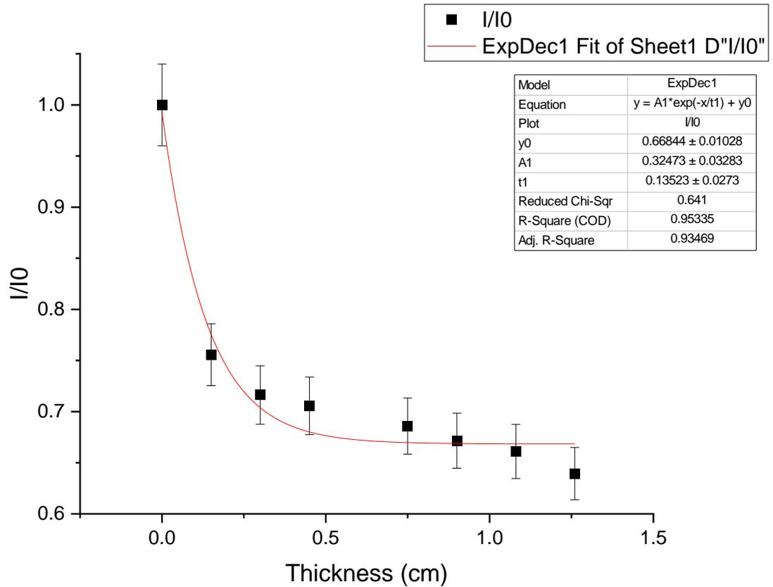
**Figure 13.** Determination of attenuation coefficient of Al
