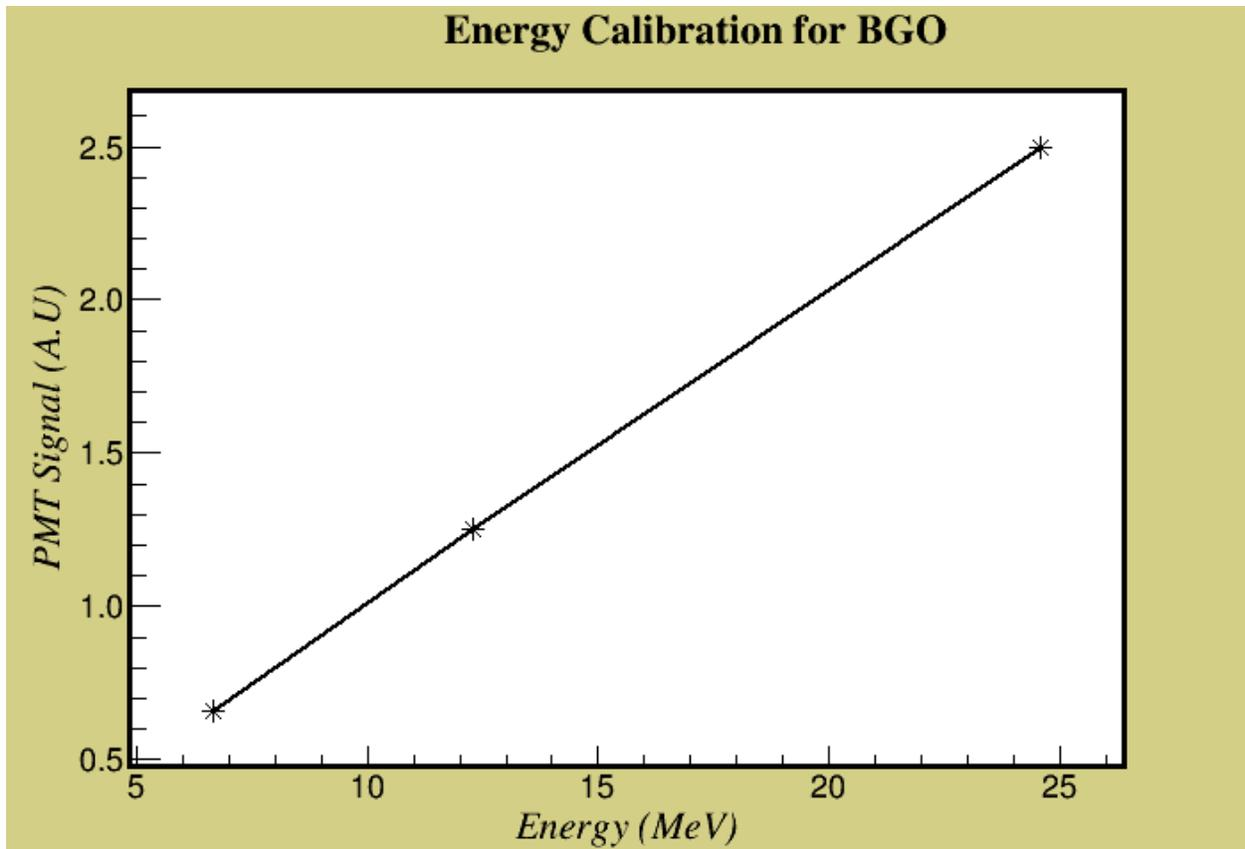
**Figure 5.** Energy calibration for BGO detector
