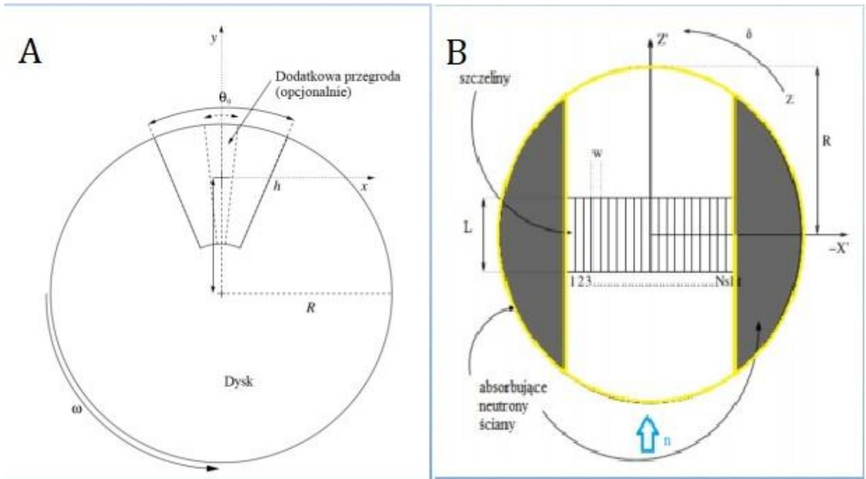
Figure 7 (a) Disc chopper (b) Fermi choppers
