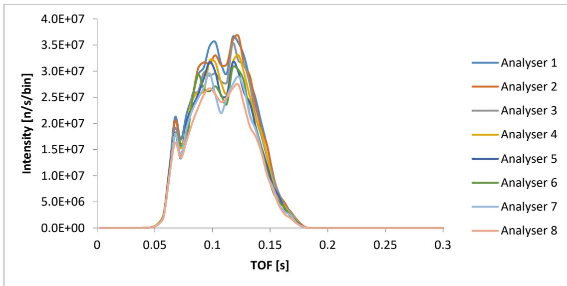
Figure 9. Time distribution from the Analyzers surrounding the sample. The TOF incident neutron spectra measured from detectors after the analyzers. The TOF scale can be easily transformed to the neutron wavelength scale using the following relation.
