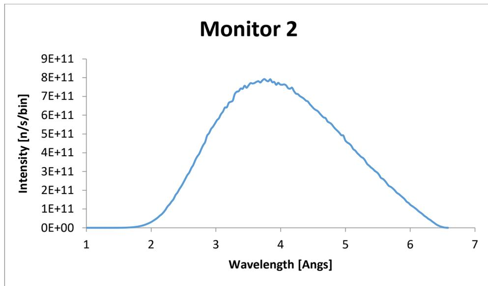
Figure 11. The wavelength distribution around  $\lambda = 3.7 \text{ \AA}$  obtained after fermi chopper
