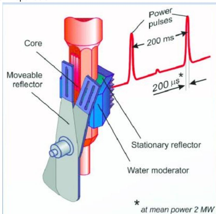
Figure 3. Pulsed neutron source.
