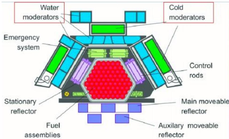
Figure 4. IBR-2 pulsed reactor
