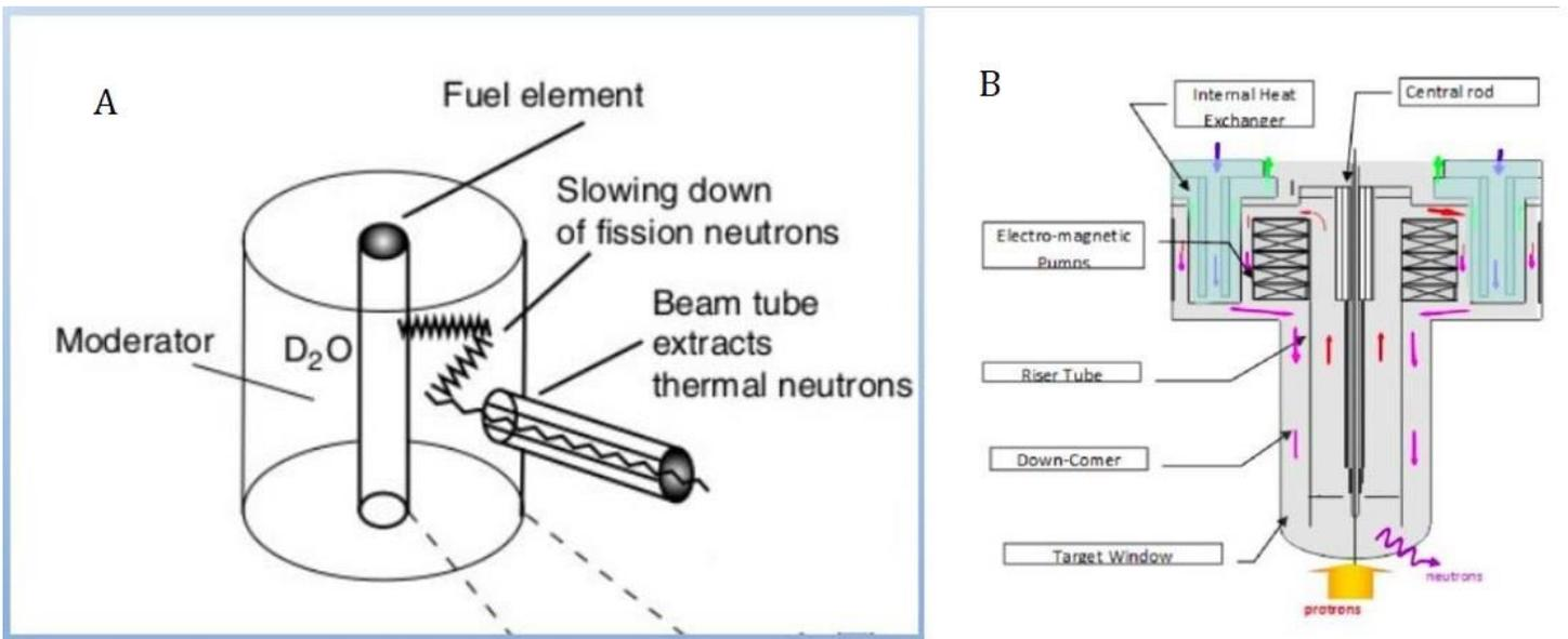
Figure 2. (a) simplified nuclear reactor showing how we can extract neutrons (b) simplified spallation source
