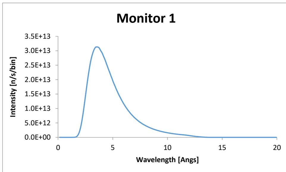
Figure 10. The wavelength distribution around  $\lambda = 3.3 \text{ \AA}$  obtained after the diskchopper
