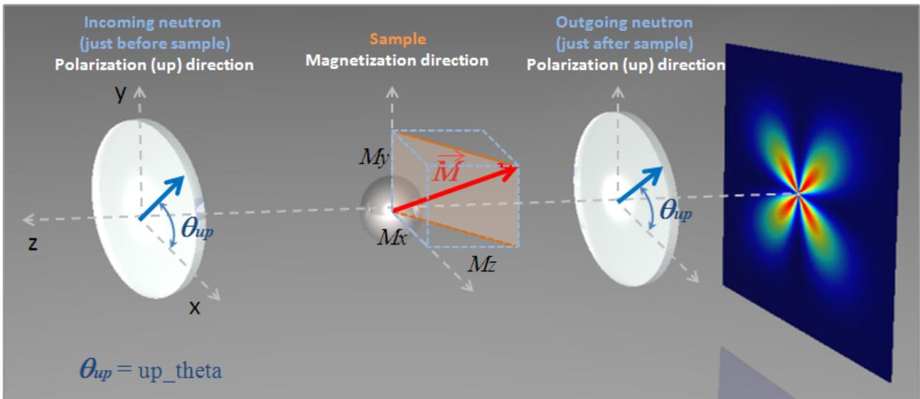
Now let us assume that the angles of the  $Q$  vector and the spin-axis ( $x'$ ) to the  $x$ -axis are  $\varphi$  and  $\theta_{up}$  respectively (see above). Then, depending upon the polarization (spin) state of neutrons, the scattering length densities, including the nuclear scattering length density ( $\beta_N$ ) are given as
