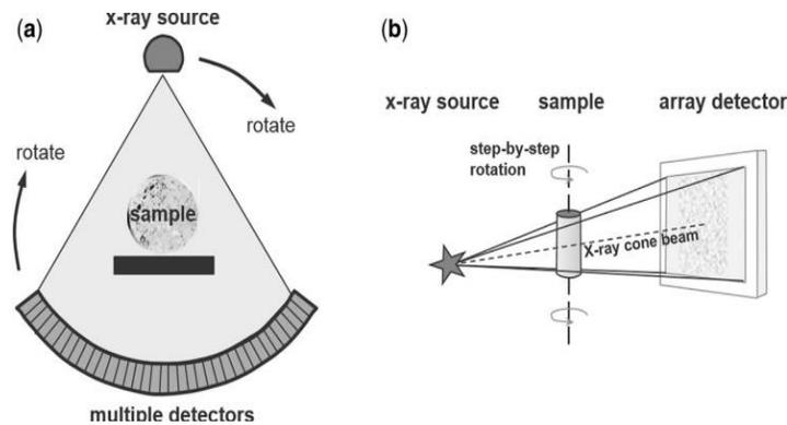
**Figure 2.** Two different configurations used in a modern third-generation CT system. (a) rotating the X-ray source and detector array, and (b) rotating only the sample under study.
