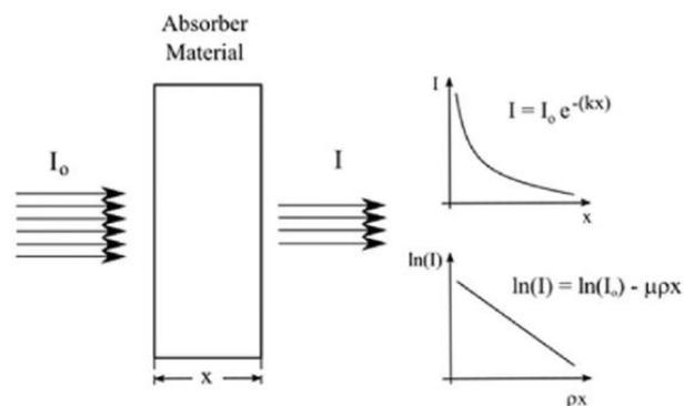
**Figure 11** Beer- Lambert attenuation law for a monoenergetic gamma ray beam of intensity  $I$  passing through an absorber of thickness  $x$ . Exponential decay representation of  $I$  versus  $x$  and of  $\ln(I)$  versus path length ( $\rho x$ ).
