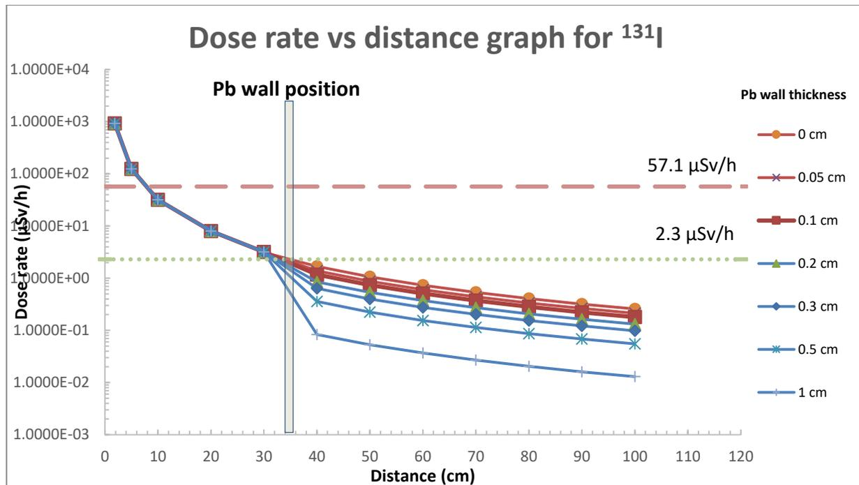
Figure 10. Dose rate vs distance graph for  $^{131}\text{I}$ .
