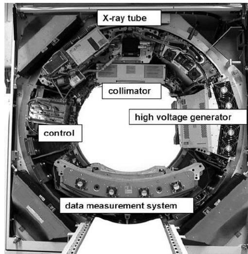
**Figure 3.** Basic system components of a modern third-generation CT system.
