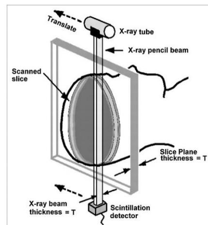
**Figure 1.** General CT arrangement for scanning the human head.
