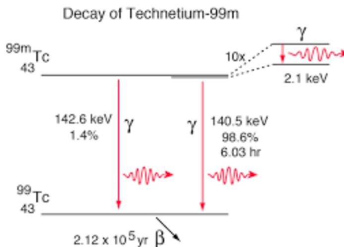
**Figure 4.** Diagram representation of the  $^{99m}\text{Tc}$  decay.
