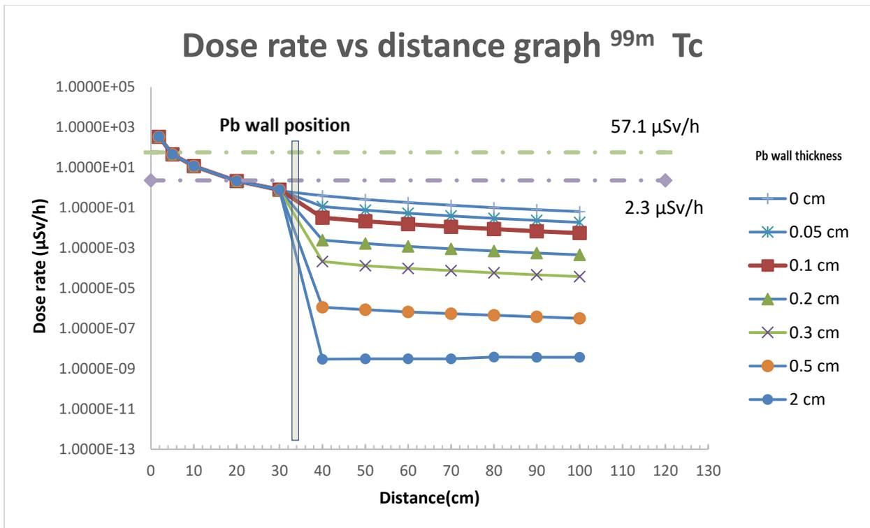
Figure 9. Dose rate vs. distance behavior calculated for <sup>99m</sup>Tc source.
