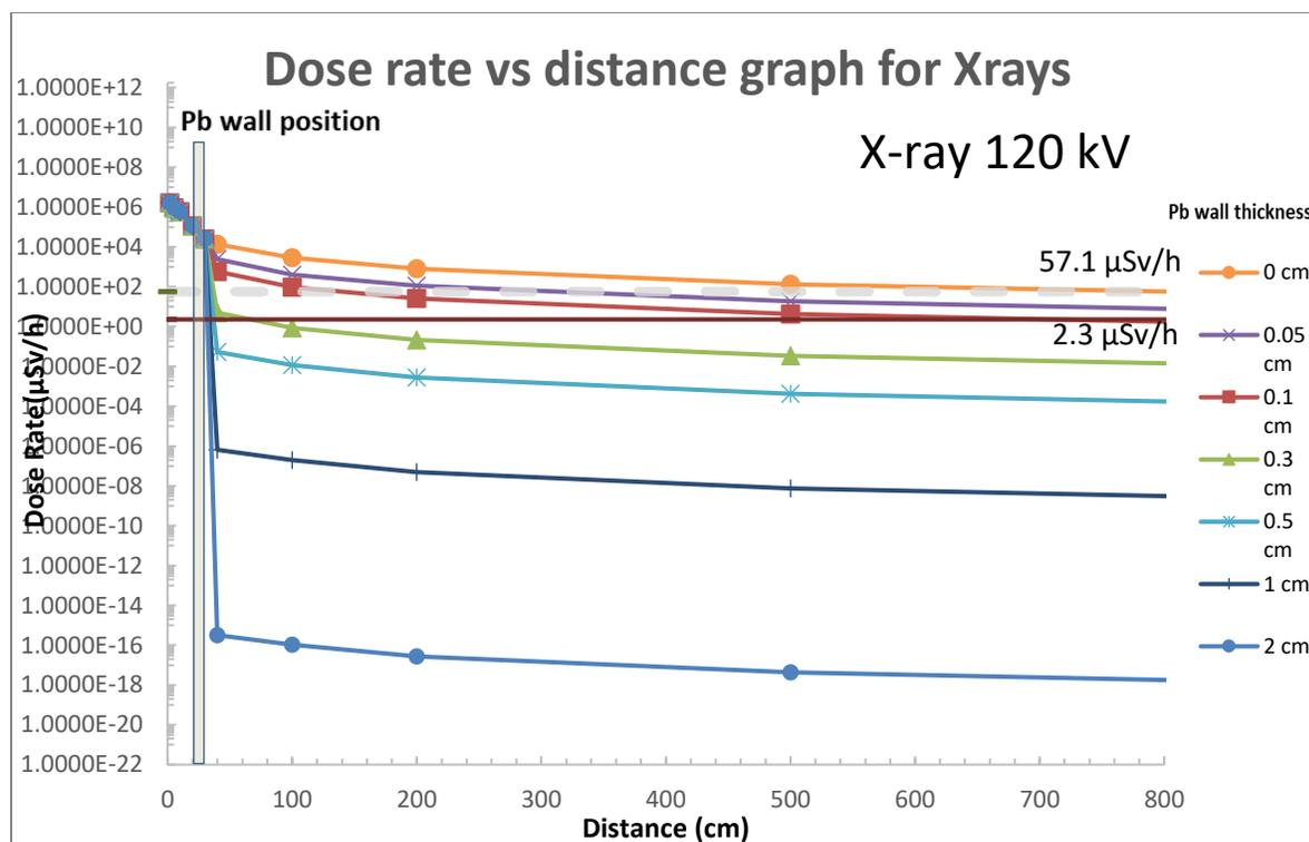
**Figure 8.** Zoom of figure 7 of dose rate vs distance graph for X-rays.
