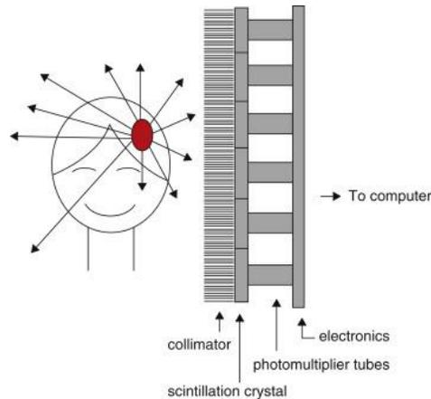
**Figure 5.** General scheme of the SPECT tomography working principle.
