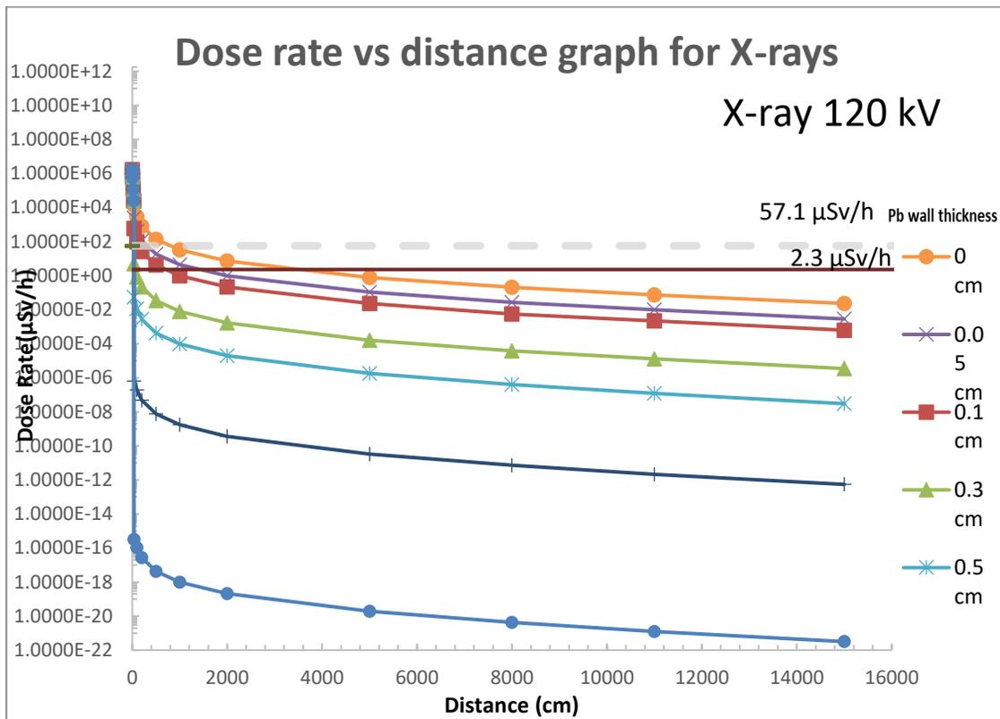
Figure 7. Dose rate vs distance graph for X-rays.
