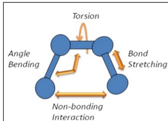
**Fig.3** Chemical bonds (bond stretching, angle bending, torsion) and non-bonding interaction
