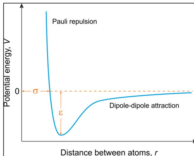
**Fig.5.** Graph of the Lennard- Jones potential function: Intermolecular potential energy as a function of the distance of a pair of particles.
