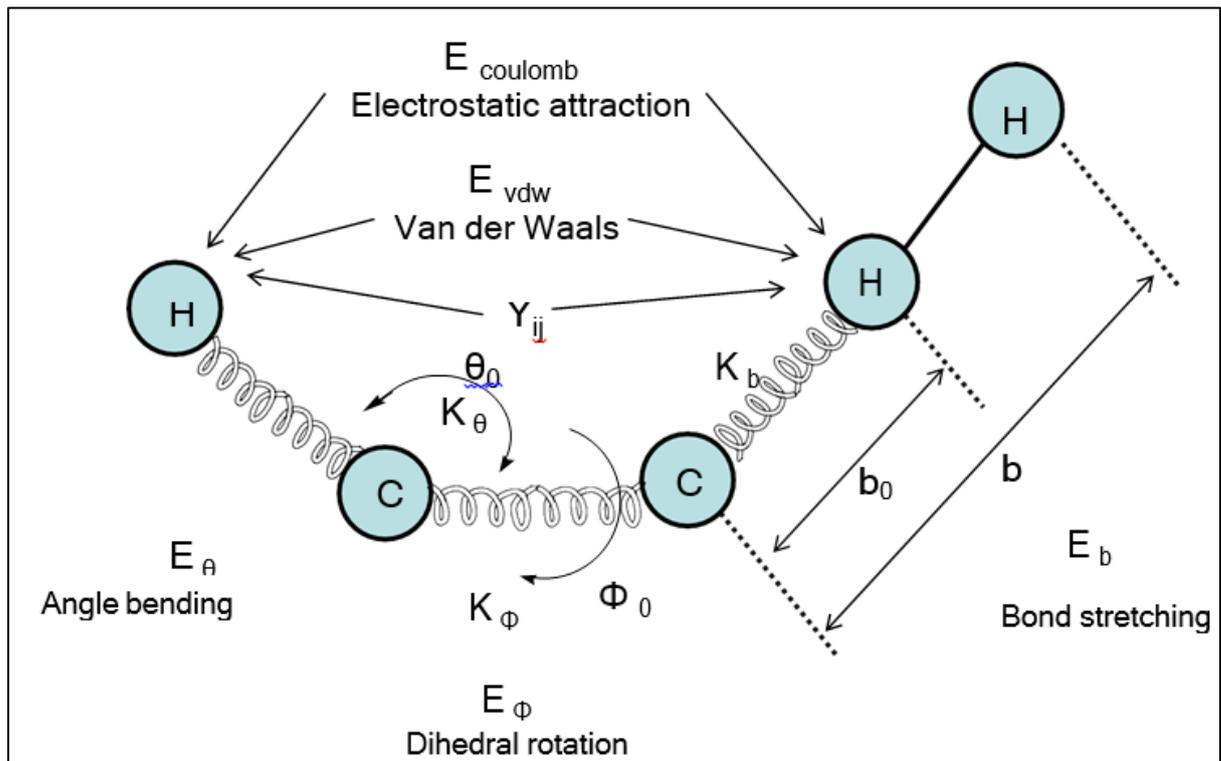
**Fig1.** Graphical representation of the bonded and non-bonded interaction and the corresponding energy terms.
