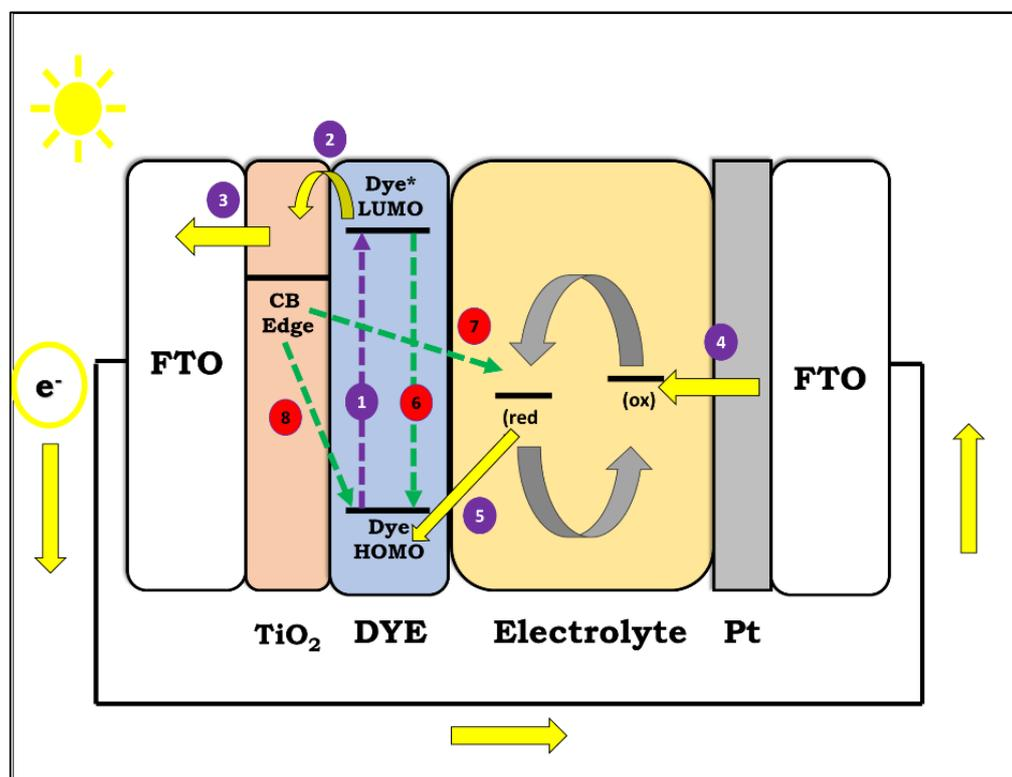
**Figure 6:** Working Principle of Dye-Sensitized Solar Cells (DSSCs)
