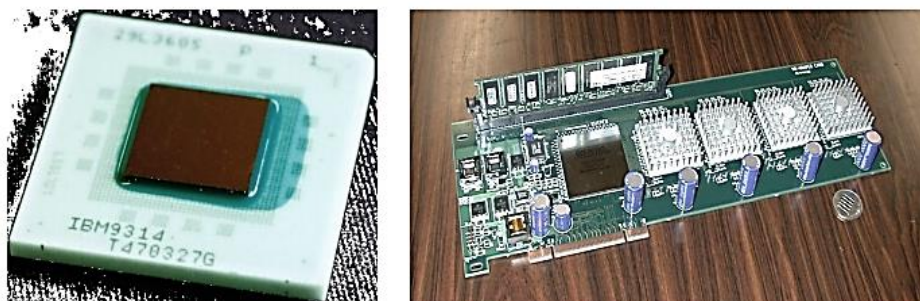
Figure 4. Special purpose MDGRAPE hardware for, among others, the correct estimation of Ewald sums
