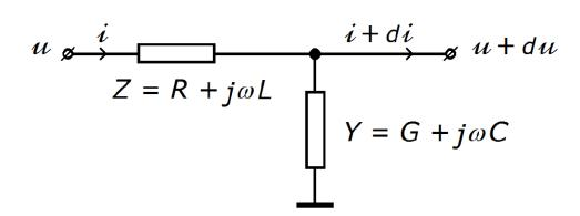
$$-\begin{pmatrix} 1 & 0\\ 0 & 1 \end{pmatrix} \partial_x \equiv \begin{pmatrix} 0 & L\\ C & 0 \end{pmatrix} \partial_t + \begin{pmatrix} 0 & R\\ G & 0 \end{pmatrix} \Big|_{\begin{pmatrix} u\\ i \end{pmatrix}}$$
