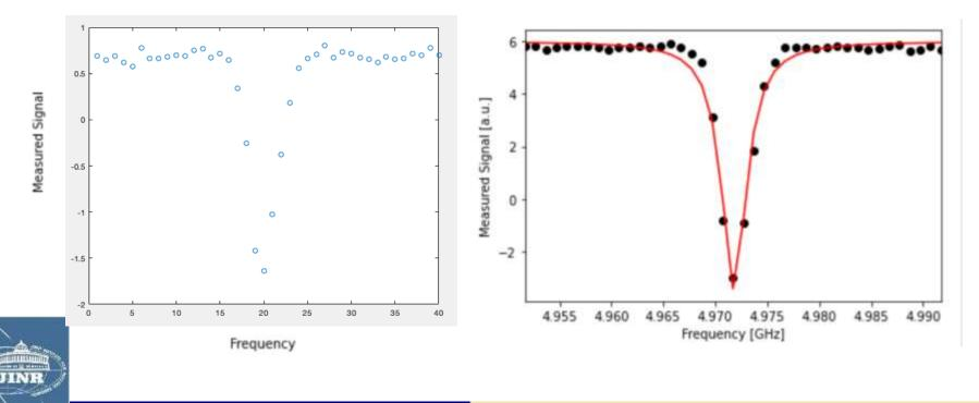
•  $\pi$ -pulse : a  $\pi$ -pulse is the pulse that "flips" the state from the state  $|0\rangle$  to  $|1\rangle$  which visualized on a Bloch sphere would be equivalent to a  $\pi$ rotation, and the strength of this pulse can be measured once the resonance frequency mentions in the Qubit frequency scan is found.
