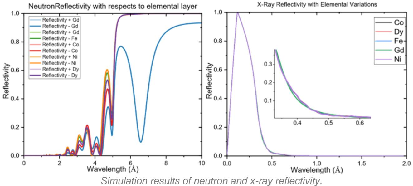
*Simulation results of neutron and x-ray reflectivity.*
