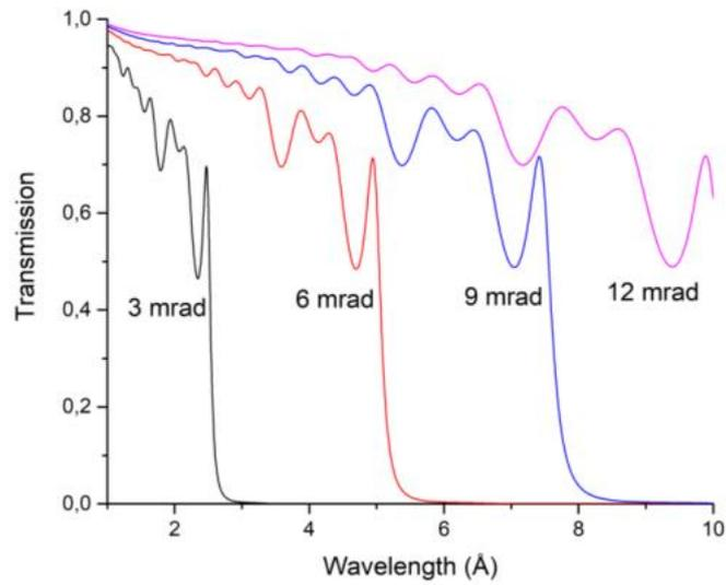
Transmission of  $\text{Al}_2\text{O}_3/\text{Nb}(100\text{nm})/\text{Gd}(3\text{nm})/\text{V}(70\text{nm})/\text{Nb}(15\text{nm})$  heterostructure for grazing angles of 3, 6, 9, 12 mrad.
