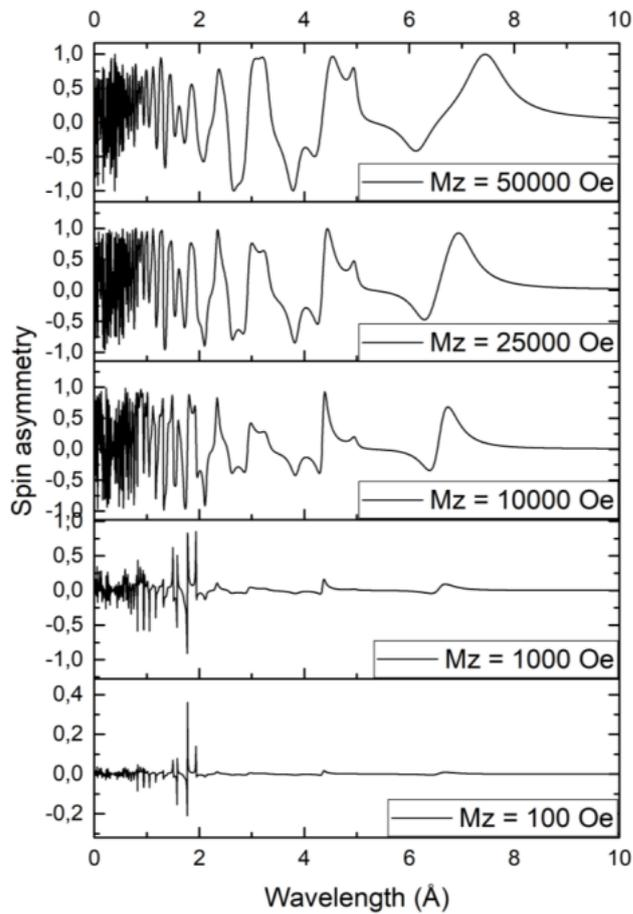
Spin asymmetry for structures in different magnetic fields with  $M_z$  of 100, 1,000, 10,000, 25,000, and 50,000 Oe.
