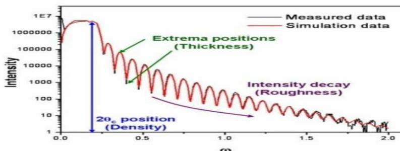
*Typical XRR pattern of a thin film on a substrate. The density, thickness, and roughness of the film are obtained from the critical angle, period of oscillations, and intensity decay, respectively*
