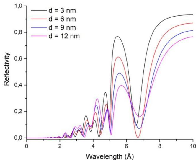
Reflectivity for heterostructure with the Gd layer thicknesses of 3, 6, 9, and 12 nm.
