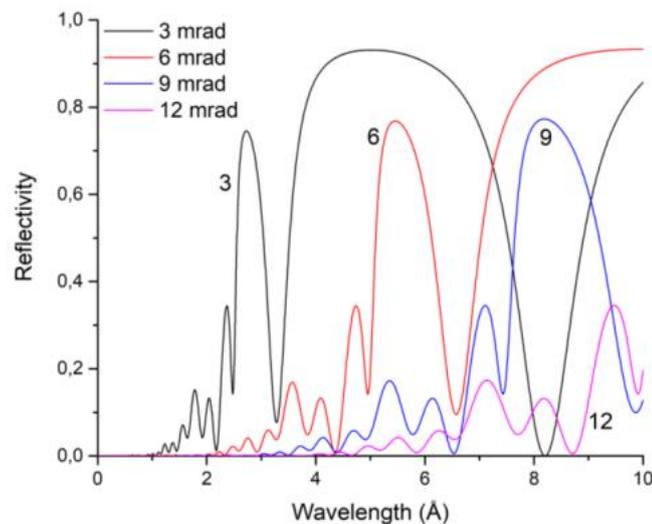
*The reflectivity of  $\text{Al}_2\text{O}_3/\text{Nb}(100\text{nm})/\text{Gd}(3\text{nm})/\text{V}(70\text{nm})/\text{Nb}(15\text{nm})$  heterostructure for grazing angles of 3, 6, 9, and 12 mrad.*
