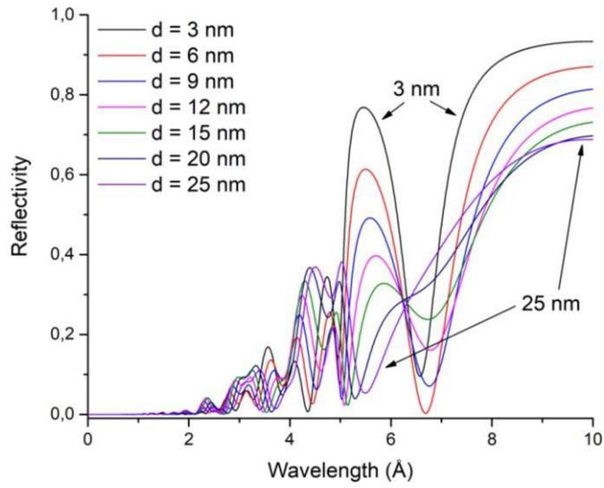
Reflectivity for heterostructure with the Gd layer thicknesses of 3, 6, 9, 12, 15, 20, and 25 nm.
