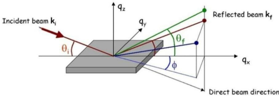
*Scheme of the neutron reflection on the sample*
