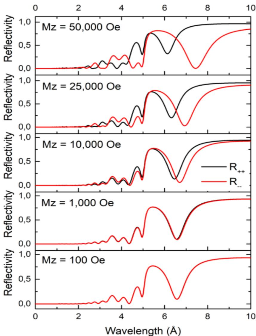
Reflectivities of the same heterostructure in different magnetizations. Magnetizations along x-axe are of 100, 1000, 10,000, 25,000, and 50,000 Oe.
